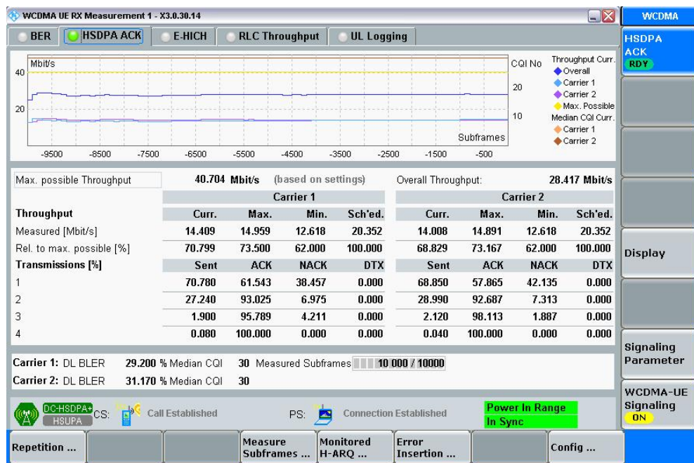
Fig. 72: WCDMA RX measurement for DC-HSPA. The measurements are adapted automatically for both streams individually and for the overall assessment.
