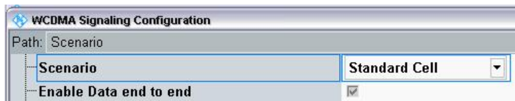
Fig. 73: Enable Data end-to-end must already be activated in the individual RANs (in this example, for WCDMA).
