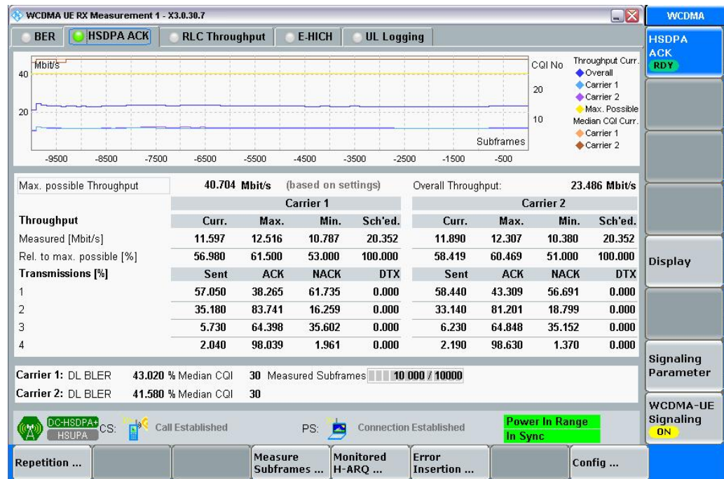
Fig. 64: WCDMA RX measurement for DC-HSPA. The measurements are adapted automatically for both streams individually and as an overall assessment.
