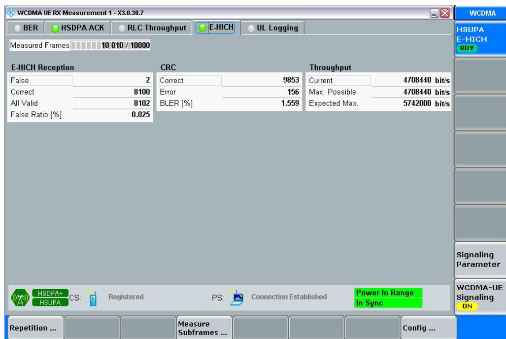
Fig. 53: W-CDMA HSUPA E-HICH measurement on HSPA channels in line with Rel 6. On the uplink channels, the CMW measures the UE's reaction to the information in the downlink channels.
