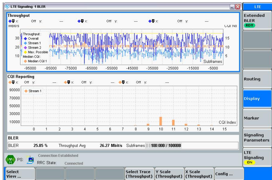
Fig. 49: LTE RX measurement for 2x2 MIMO. The measurements are adapted automatically for both streams individually as well as in the form of an overall assessment.
