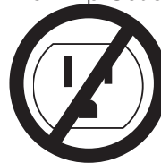
Wrong 15 Amp Outlet
