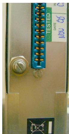
When mounted in the AMS Neve rack, these pre-sets are accessed by removing the rack rear panel and can be adjusted through the rear connector mounting panel.
