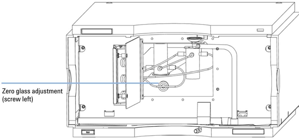
**Figure 34** Turning the zero glass adjustment screw
