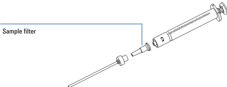
**Figure 33** Syringe with Sample Filter
