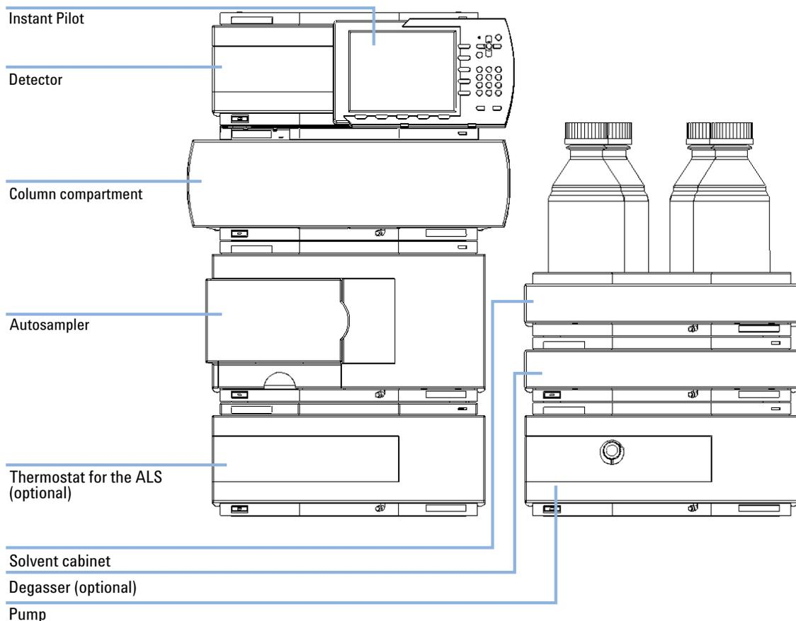
**Figure 18** Recommended Two Stack Configuration for 1260 (Front View)
