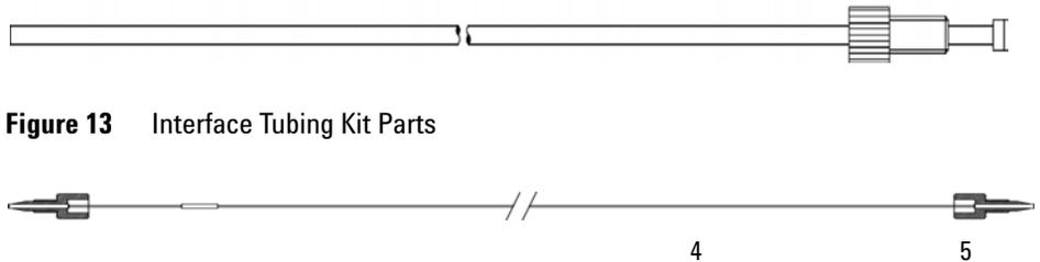
**Figure 14** Interfacing Capillary Parts
