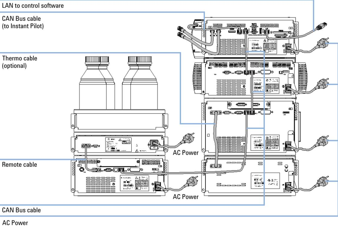
**Figure 19** Recommended Two Stack Configuration for 1260 (Rear View)
