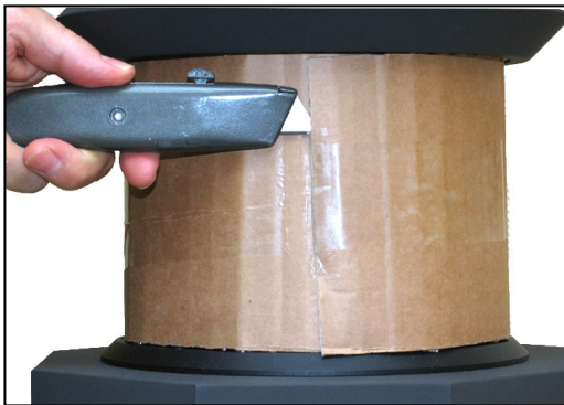
Figure 8. The Correct Way to Remove the DDD Driver Cover
