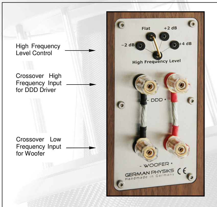
Figure 7. Input Terminals and Crossover Adjustment
