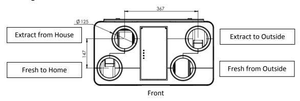
**Inverted Configuration:** (Factory Set: Must be specified at time of order)
