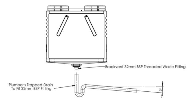
The condensate drain should incorporate a "P Trap" or equivalent, as shown, before being discharged into the waste drainage system of the dwelling. The "P Trap" should be filled creating an immediate seal upon installation.
