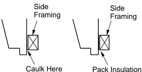
**Figure 34 - Sealing Between Appliance and Framing**
