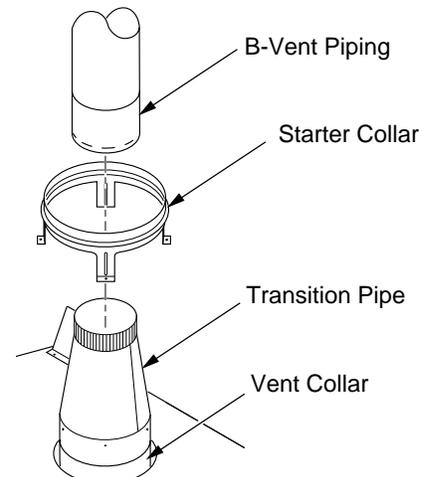
Figure 9 - Installing Transition Pipe and Starter Collar
