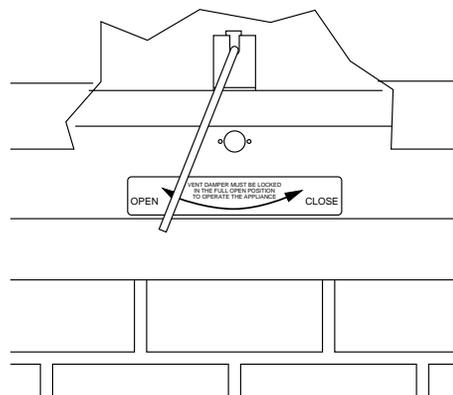
**Figure 38 - Opening Vent Damper**
