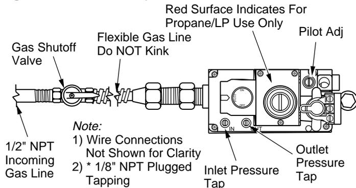
**Figure 21 - Connecting Flexible Gas Line to Millivolt Valve**
