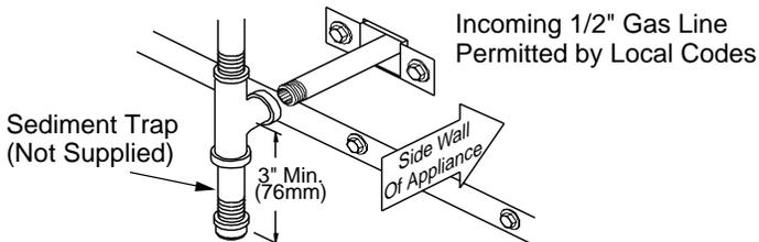
**Figure 20 - Sediment Trap**
