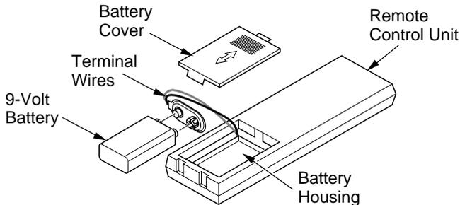
Figure 17 - Installing Battery in Hand-Held Remote Control Unit
