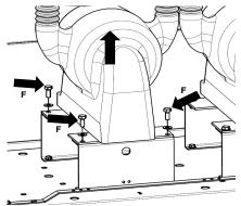
Replace the VTs (12 HM6 screws F).
