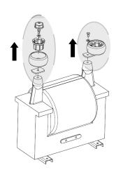
Disassemble the distribution frames and replace the VT.
