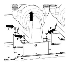
Unscrew the M8 front and rear screws F holding the VT support in place. Extract the assembly.
