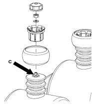
Unscrew the M8 nut to remove the distribution frame
