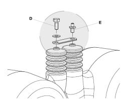
Unscrew the M8 screw D and the special screw E to remove the strip connecting with the primary terminals.
