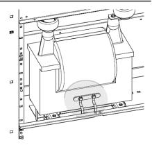
Unscrew the earth busbar metal foil
