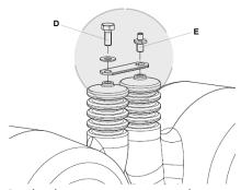
Put back strip connecting with the primary terminals, the primary connections D and the distribution frames E.
