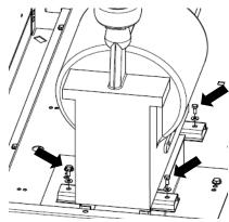
Remove the 2 HM8 fastening screws.
