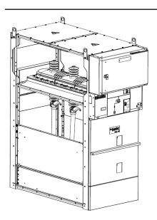
Reassemble the VT set in the cubicle, proceeding in opposite order to disassembling. HM8 screw tightning torque: 2.2 Nm.
