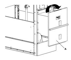
Remove front panel A. Remove the HV fuses (see user manual).
