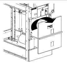
Remove the front panel Remove the HV fuses (see user manual).
