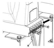
Disconnect the secondary circuits of the VTs 3 M6 screws.
