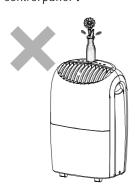
Do not cover all the air outlets of the machine  ${\tt !}$
