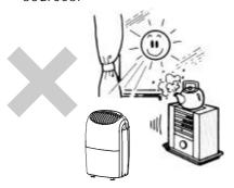
Do not use insect, oil or paint spray around the Machine, it might cause damage to the plastic parts or start a fire.
