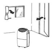
When moving or put in storage, do not place the dehumidifier on side way or upside down and avoid violent shaking.
