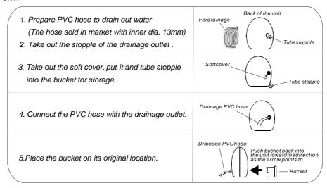
2) Put the water tank back, do according to the instructed way.
