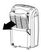
B. Clean the filter by vacuum cleaner or washing with clean water then dry the filter using dry cloth.
