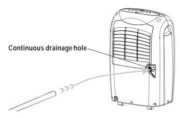
1) Put in the PVC hose into the back of the closed hole, then connect the PVC hose to the front.
