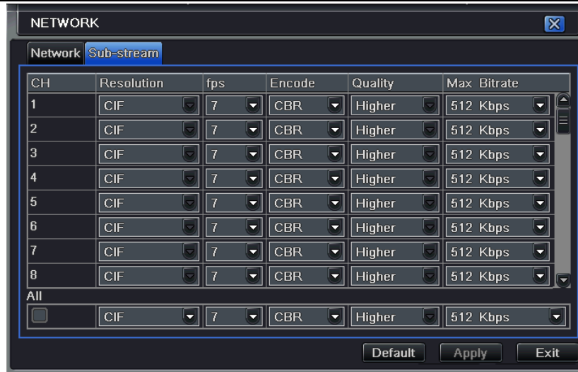
Fig 4-33 network configuration-sub stream
