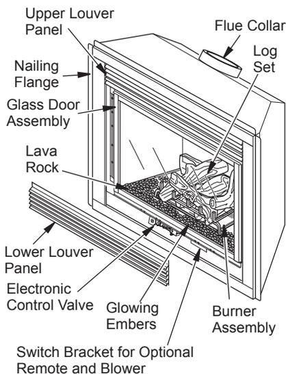
**Figure 1 - Direct-Vent Fireplace with Millivolt Ignition**
