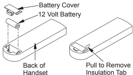
**Figure 41 - Installing Battery into Back of Handset**
