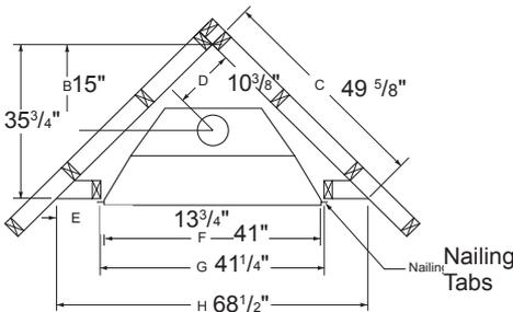
**Figure 5 - Framing Clearances for Corner Installation**
