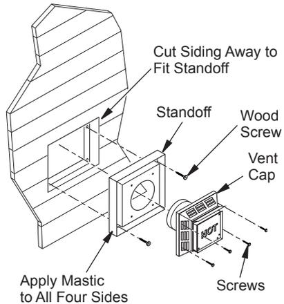
**Figure 11 - Installing Siding Standoff (Combustible Exterior Wall)**
