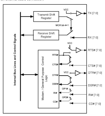
The line test contains a test of all modem lines, as you can see RTS and CTS, DTR and DSR, OP1 and RI and finally OP2 and CD. Only the static states for both electrical levels are tested on each sender – receiver line pair.
