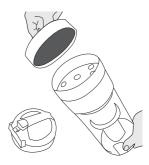
Wash both filter and sponge under warm water until the water runs clean. Remove excess water by shaking and leave to dry for 24 hours. Reassemble and refit filters to cleaner, only when they are completely dry.
