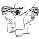
Rotate the brush to ensure free movement of the belt.
