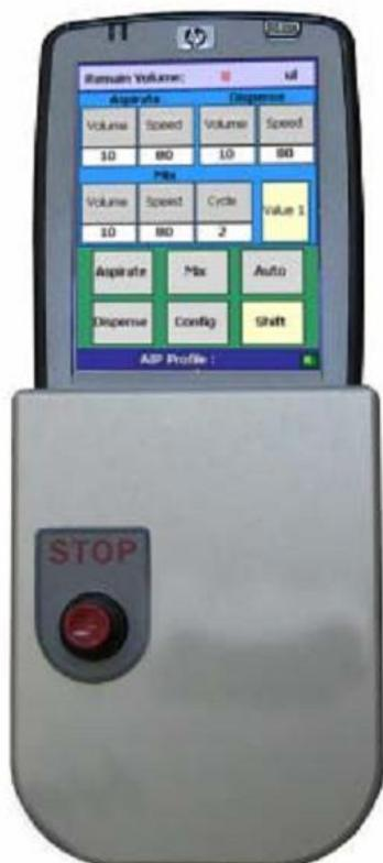
For emergency stop at any time, press the STOP button on the PPC controller.
