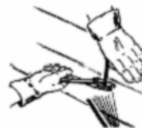
When cutting horizontally tensioned strapping, stand to the left of the cut, hold the strapping against the package, and cut to the right of the hold.
