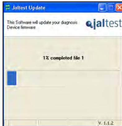
Once the last file has been loaded and in order to finish the update process, the program will ask to introduce a name for identifying your Jaltest device. Then press 'Accept' and the update process will have finished successfully.
