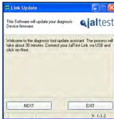
b) Update. After deleting the Jaltest memory, the update process begins. It is necessary to install three files. This process is automatic. The screen shows the update progress and the file which is being installed.
