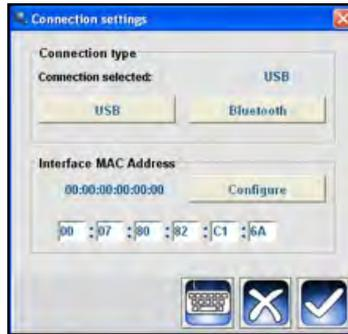
With this option you can set the type of connection with the interface, whether it is via Bluetooth or via USB. Besides you can also set the MAC address.
