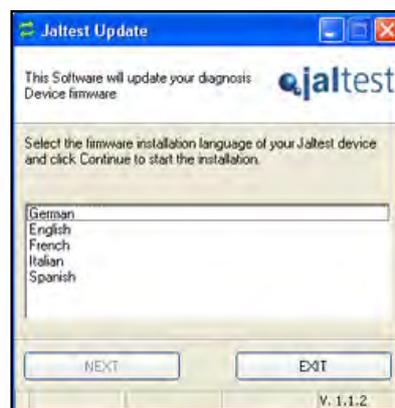
The update process for this tool takes approx. 45 minutes. Connect your USB device, switch it on and select 'JaltestSoft' (option number 4 in the main menu). Press 'Next' to continue.
