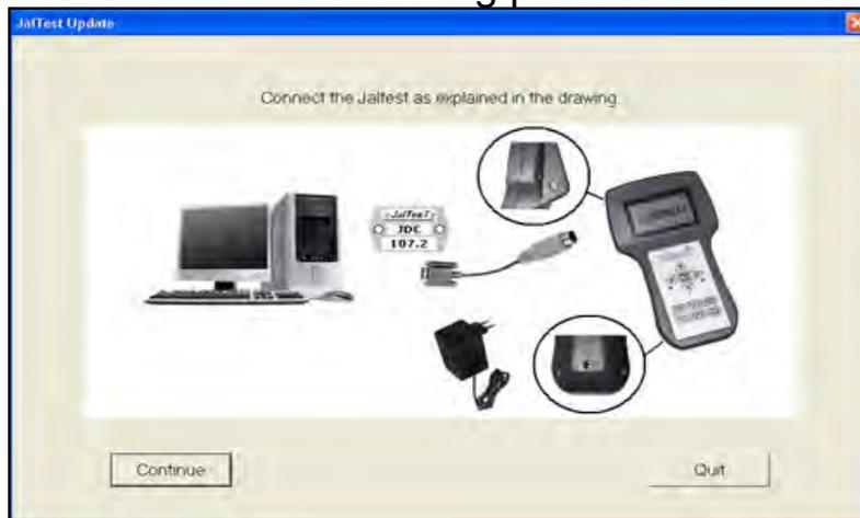
Select the COM port of your PC which has been used to connect the update cable and press 'Accept'.
