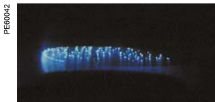
Fig. 3: diffuse vacuum arc AMF technology
