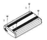
B. Loosen the four screws on the surface of the unit.
