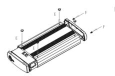
E. Reverse the procedure by re-inserting the bracket to the aluminum casing and securing all the screws that was previously removed.Congratulations, you have completed the hardware installation
