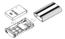
C. The plastic bracket should slide out effortlessly. Insert your hard drive, connect the IDE and power cable from the enclosure accordingly.Please ensure that your hard drive jumper setting is configured at Master.
