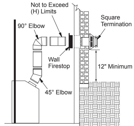
**Figure 15 - Horizontal Termination Configuration for Corner Installation Using One 90 Degree Elbow**
