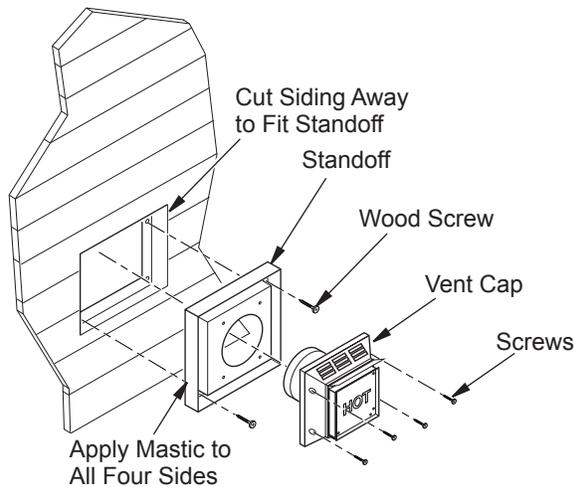
**Figure 11 - Installing Siding Standoff (Combustible Exterior)**
