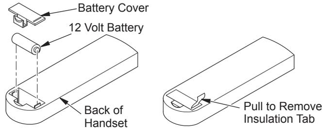
**Figure 48 - Installing Battery into Back of Handset**
