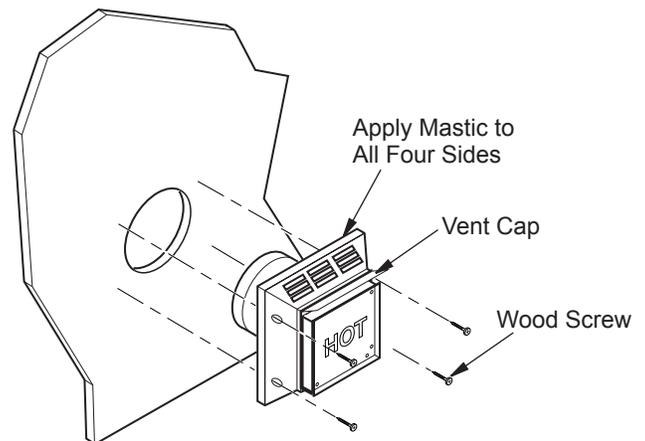
Figure 10 - Installing Horizontal Vent Cap (Noncombustible Exterior)
