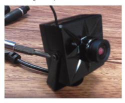
b) Secure the camera's mounting bracket in the desired location using the wall mount bracket and screws provide as shown on below.
