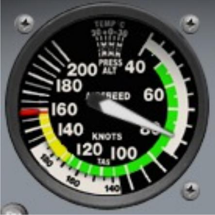
**Figure 2.11:** The airspeed indicator in the Cessna 172
