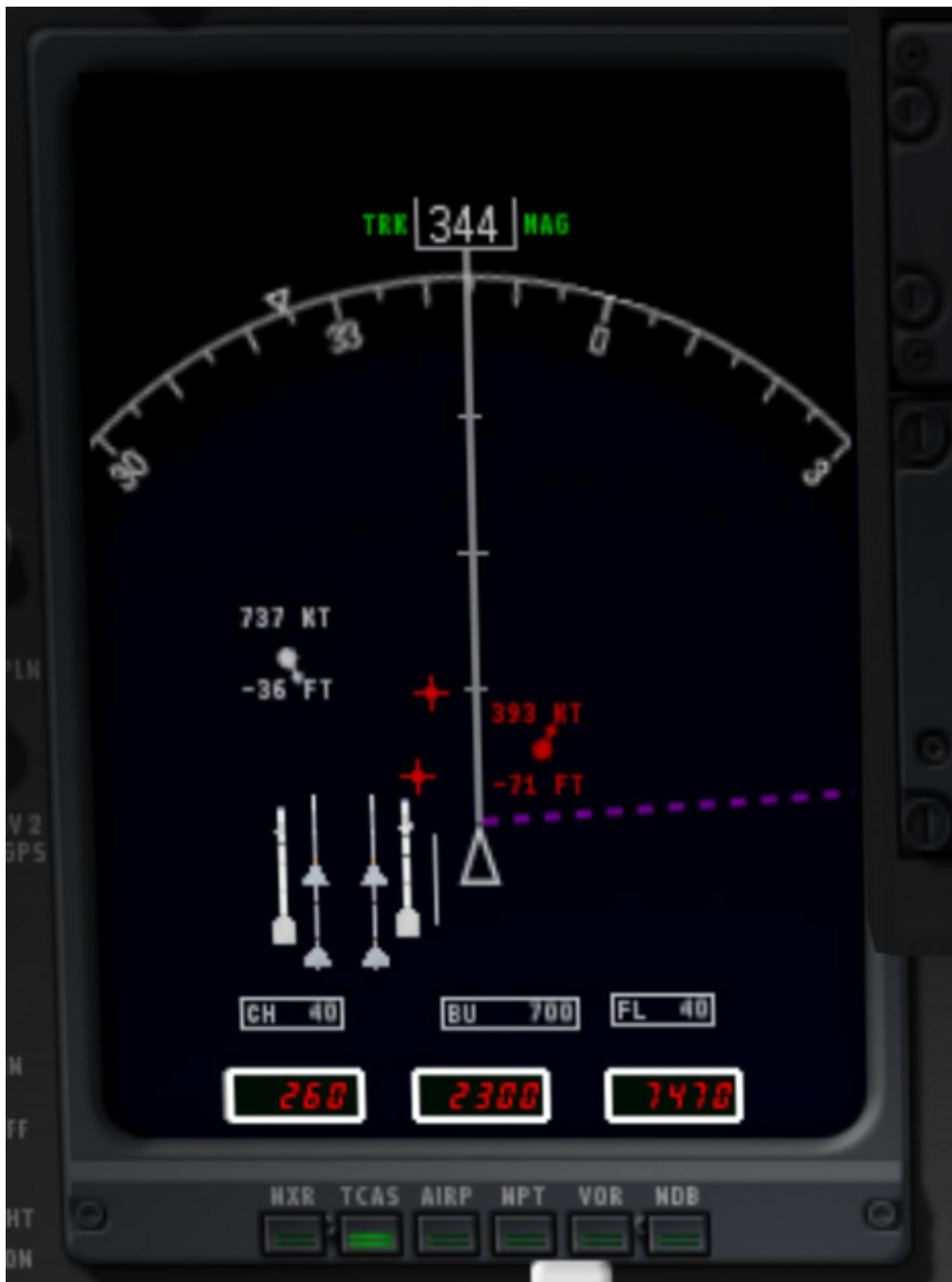
**Figure 8.9:** The moving map display with a target selected, located about 30 degrees to the right, in front of the aircraft and travelling at 393 kts
