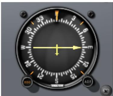
**Figure 7.1:** The ADF in the Cessna 172
