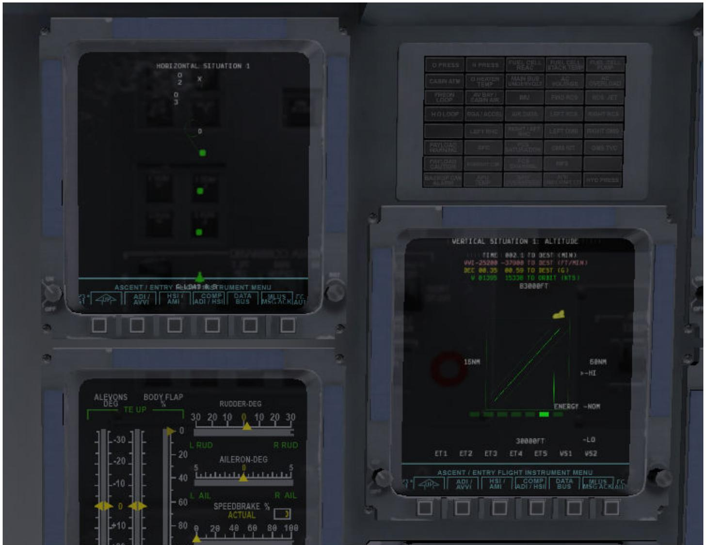
**Figure 8.1:** The space shuttle's horizontal and vertical course displays
