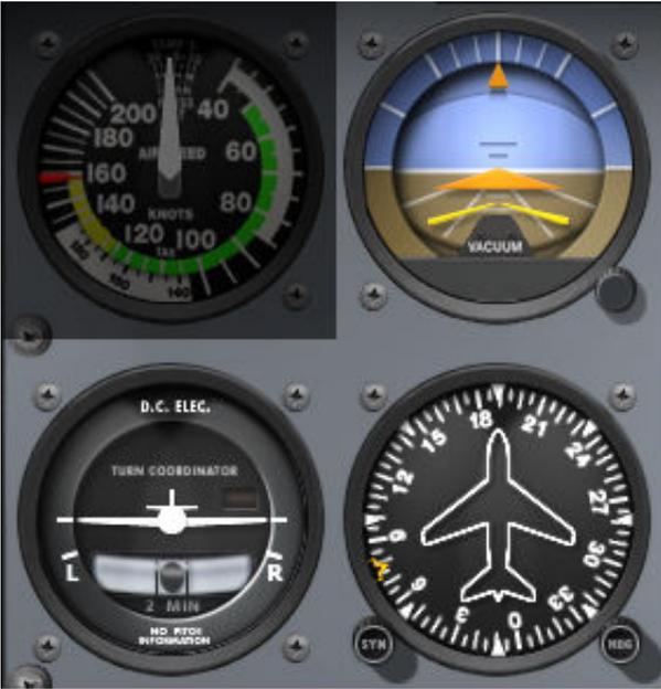
**Figure 7.4:** The three primary gyroscopic instruments in the Cessna 172
