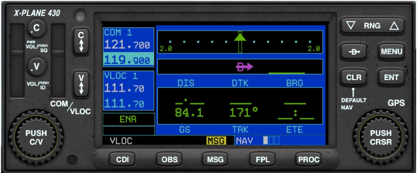
**Figure 7.5:** The X-Plane 430 GPS navigator in the Cessna 172.
