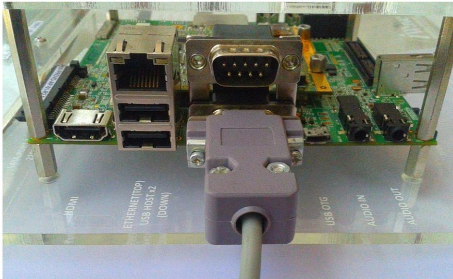
**Figure 2: Debug UART connection**
