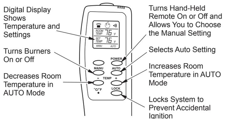
Figure 54 - Thermostat Hand-Held Remote Control Unit GHRCTB
