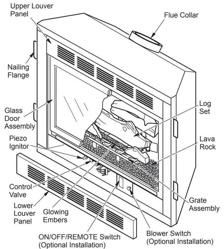
Figure 1 - Direct-Vent Fireplace with Millivolt Ignition
