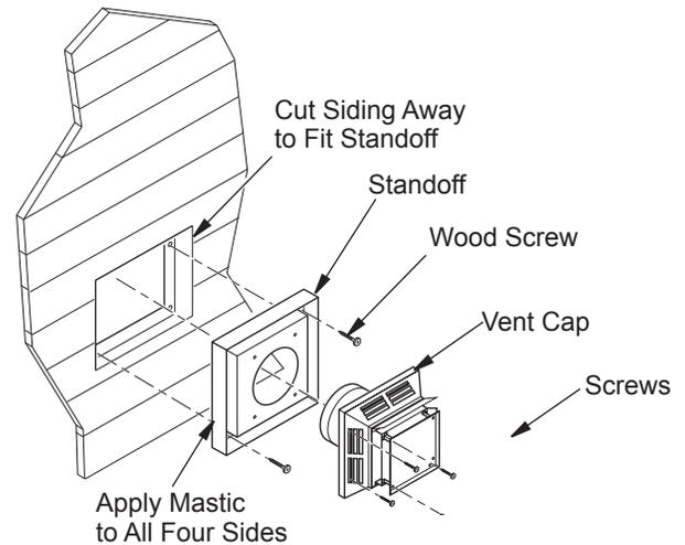
Figure 11 - Installing Siding Standoff (Combustible Exterior Wall)
