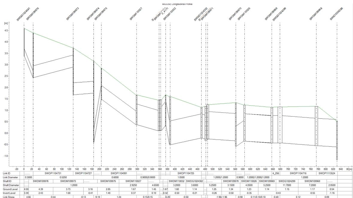
**Figure 7 Long section 1 with non-critical errors resulting in negative slopes.**
