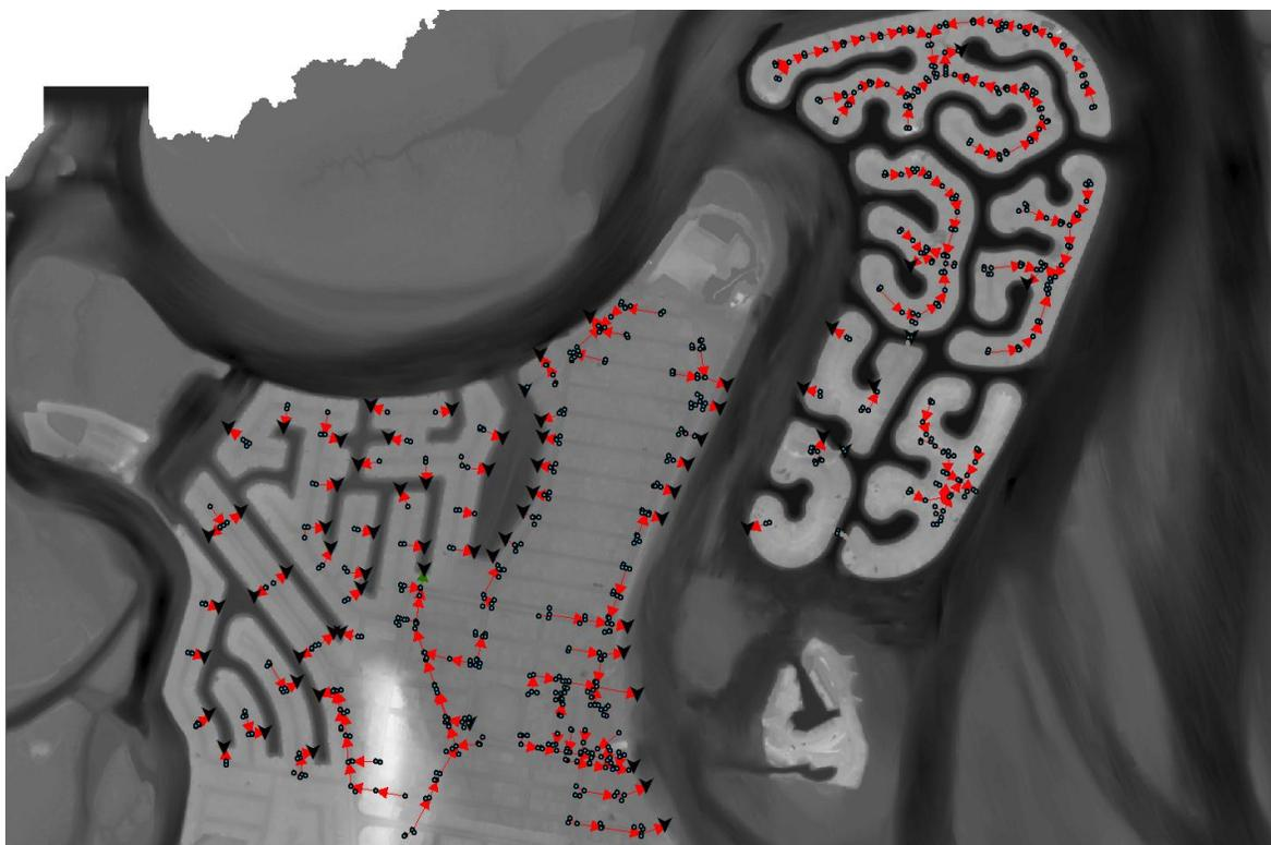
**Figure 9 Paradise Point Hope Island model network and bathymetry after manual clean-up.**
