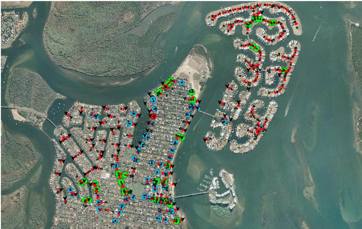
**Figure 6 Paradise Point, Hope Island model, symbolisation of model data errors prior to any manual clean up being undertaken.**
