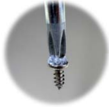
Attach screw to screwdriver
