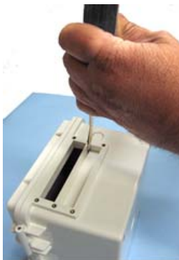
Accessing secondary cable slot
