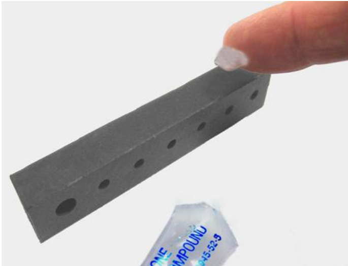
Greasing the cable channel
