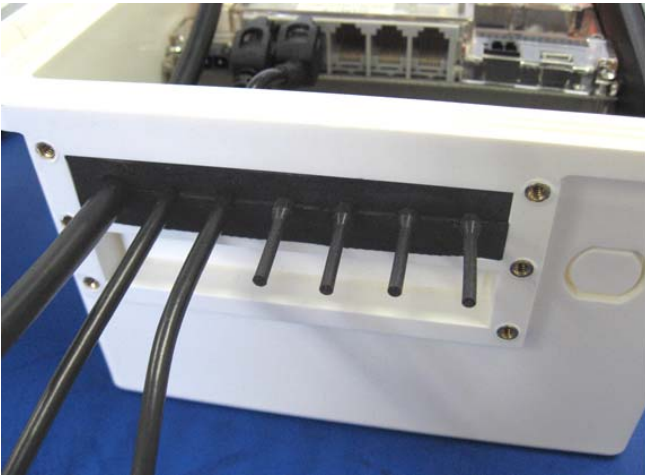
Channel pressed into case
