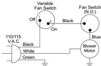
*Figure 29 - Blower Wiring Diagram for Thermostat-Controlled Models*
