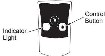
**Figure 52 - On/Off Hand-Held Remote Control Unit HRC100**
