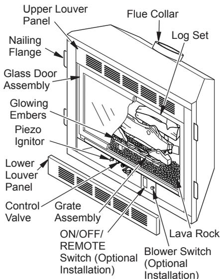
Figure 1 - Tudor Direct-Vent Fireplace with Millivolt Ignition
