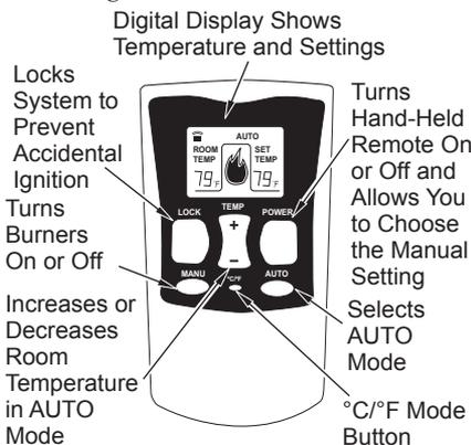
**Figure 53 - Thermostat Hand-Held Remote Control Unit HRC200**
