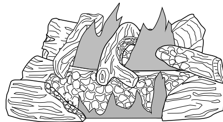
Figure 51 - Typical Flame Pattern
