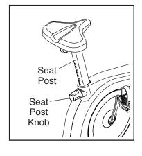
the knob is engaged in one of the adjustment holes in the seat post. Then, turn the knob clockwise to tighten it.
