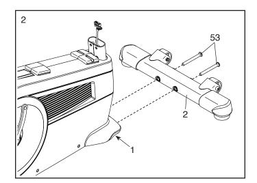
3. Attach the Rear Stabilizer (3) to the Frame (1) with two M10 x 110mm Screws (53).
