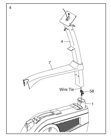
5. **Tip: Avoid pinching the wires.** Slide the Upright (4) onto the Frame (1). Attach the Upright with four M10 x 15mm Screws (65) and four M10 Washers (31); **start all four Screws, and then tighten them.**
