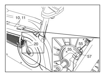
Next, rotate the Left Crank Arm (20) until a Magnet (55) is aligned with the Reed Switch (57). Slide the Reed Switch slightly toward or away from the Magnet. Then, retighten the ST4.2 x 19mm Screw (35).
