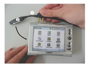
The FM remote is hot pluggable. You do not have to shut off the AV300 in order to plug in the FM Remote control or remove it. First, (1) plug in the doublejacks and then (2) attach the mini-centronics connector. Now plug your headphones into the FM Remote Control itself.
