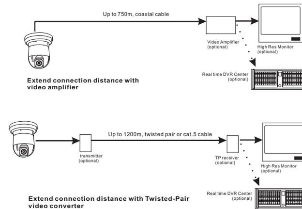
Extend connection distance with Twisted-Pair video converter
