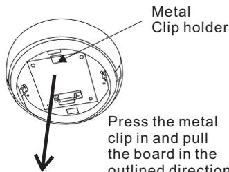
Press the metal clip in and pull the board in the outlined direction.
