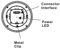
Once the base board is connected to power, the power LED will light up.
