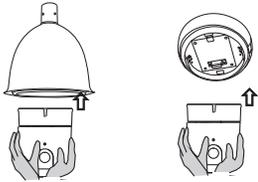
Installing the core unit by inserting it into the housing. Please note the position of the connector. For releasing, please press the lever-lock to core and pull off the unit.
