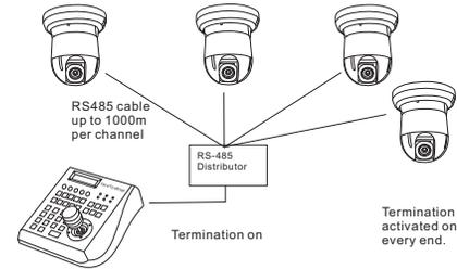
The advantage of star-connection is that every channel can work independently and supports a cable length up to 1000 meters (depending on the quality of the cable). In case more dome cameras are installed, the star-connection can be extended with additional RS485 distributors.
