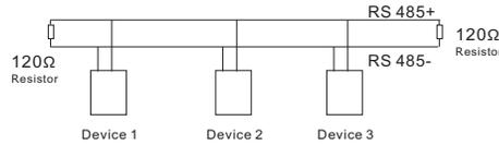
The speed dome series provide an integrated termination switch. It should be turned ON on the dome serving as the last device. If a controller keyboard is used, you also need to turn the termination ON on the keyboard. Please refer to the keyboard's manual for details.
