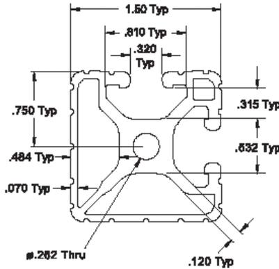
**1502 T-Slotted Extrusion Machining Services**
