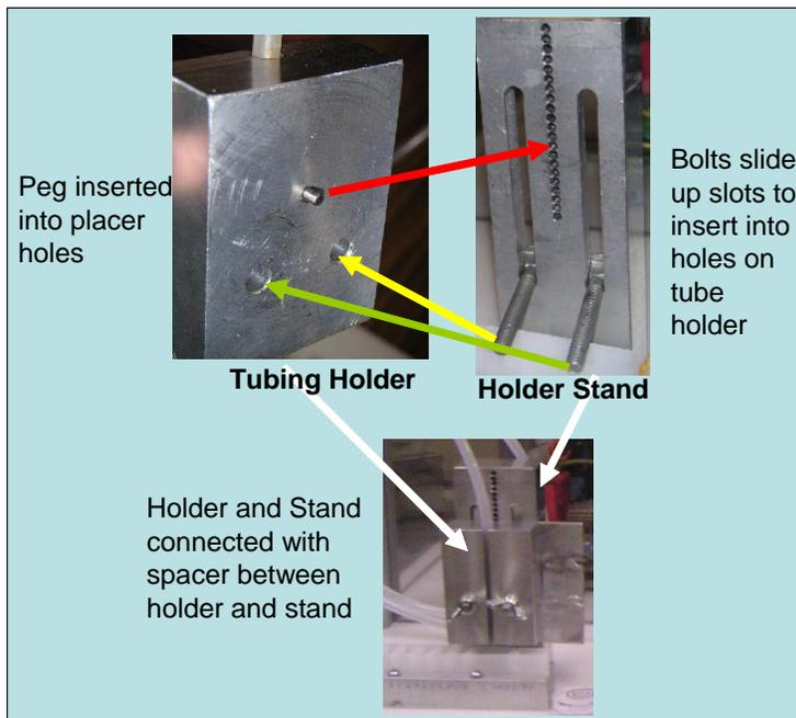
**Figure 8: Tubing Holder and Stand**
