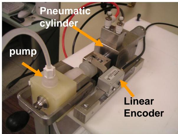
**Figure 2a: Pneumatic driver and pump**
