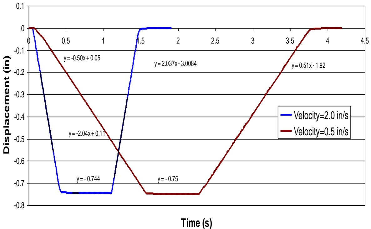
be a result of the imperfect coupling between the driver and the pump, which will allow the driver to move slightly before the pump begins to move. Since the linear encoder is
