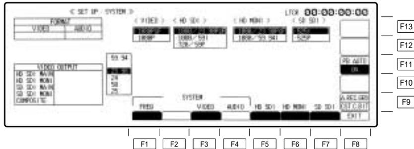
The frequency setting is possible when the F1 key is pressed. Select the frequency by cursor keys [▲, ▼] and press the ENT key, then the frequency is secured. In 59 Hz mode, the selection window will be further displayed (1080i/525i/720p). Select the format by the cursor key, and press the ENT key to secure the format. Then, select its 4-channel or 8-channel audio version, and enter the format by pressing the ENT key.
