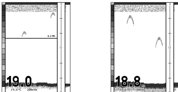
Fig. 6.3.1.1 - Example of 200kHz (left) or 50 kHz (right) Fish Finder Full display
