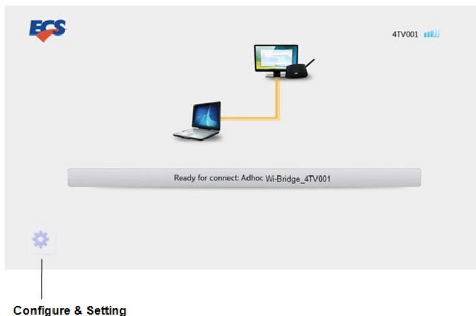
The default setting will be **“AP mode”** when use Wi-Bridge for the first time. If you want to make the Wi-Bridge device connect to the wireless network, you can use the Remote Controller to configure the wireless network or use wireless mouse on Wi-Bridge to set the configure on LCD TV directly. For more detailed information, please refer to the **“Wireless Network Configuration”** (page 11) section.
