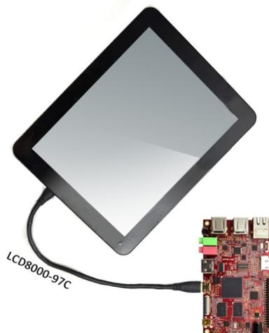
**Figure 1** Connections between RIoTboard and LCD8000-97C
