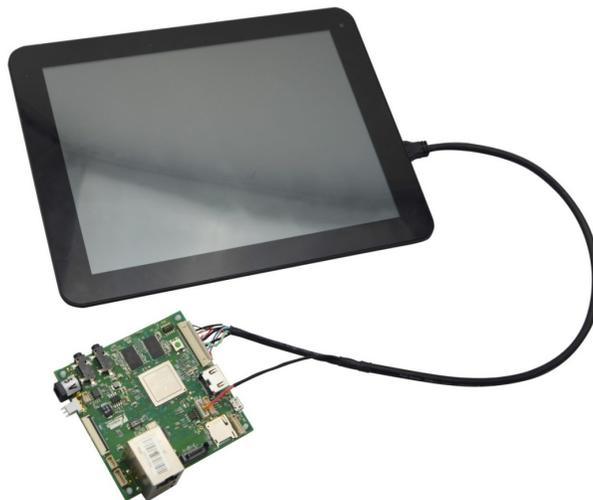
**Figure 4** Connections between SABRE Lite and LCD8000-97C
