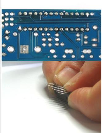
Now it is time to insert the chip! Carefully remove it from the packaging. You'll have to bend the pins in a little to make them fit nicely into the socket. I grab both ends and rock the pins against a tabletop. (The image shows a smaller chip, but the idea is the same). Once the legs are parallel, locate the Ushaped notch in one end. Make sure that this end goes into the notched-end indicated on the silkscreen (and, hopefully, the socket as well)
