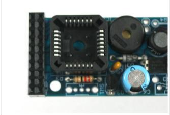
Next place the 2x10 0.1" spacing female header. it goes with the socket facing up.
