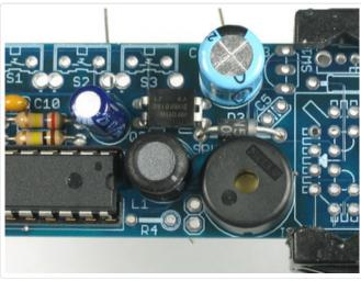
Next is the inductor **L1** which stores and releases power to boost the voltage up. Inductors are just coils of wire so they are not polarized and can go in either way.
