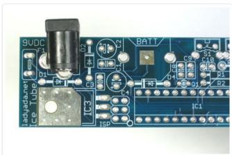
The first part to be placed is the DC jack. This connector allows you to power the clock using an external power adapter.
