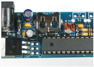
Solder in the final Schottkey diode (D4), this one keeps the battery disconnected until the main power dies. Place it so that the stripe is on the left hand side. Solder and clip the diode.
