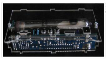
Place the back onto the kit, aligning the holes and enclosure guides.
