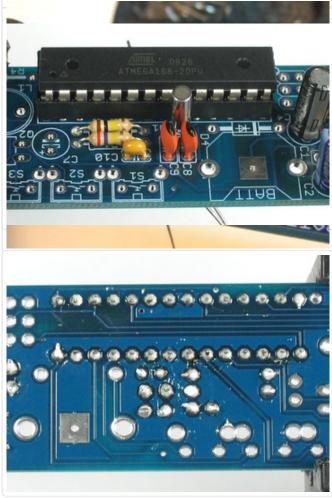
Now we will place the 32.768 khz clock crystal. This crystal lets the chip keep time properly. The crystal **Q1** is a silver tube and is symmetric so it can go in either way. Next to it goes two 20pF capacitors **C8** and **C9**. These caps stabilize the crystal to keep the timing correct. They are ceramic capacitors but are in a disc package. They are symmetric and can go in either way.
