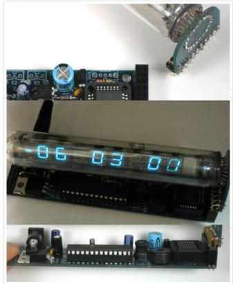
Clear off your desk and plug in the DC adapter. You should hear a beep and the display turn on and display some numbers (probably 12 00 00) If you get anything on the display you're doing great and the tube is working well. **Note that it will be very dim!** That is because the display is designed to be at the lowest brightness (voltage) when first built. Once its in an enclosure you can make it brighter! If the tube seems to not be working, turn off all the lights and look again.
