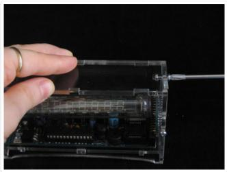
Slide the top piece so that the hex nuts align with the T-slots and screw it into place.
