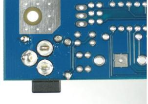
Next it is time to clip the extra long leads of the diode. Using your diagonal/flush cutters, clip the wires right above where the solder joint tapers off.
