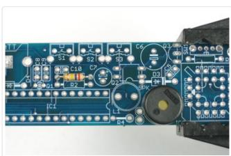
We will now continue and place the 270K resistor **R1**, this resistor is part of the 'lost power' detection circuitry. Resistors are nonpolarized so they can go in 'either way'. Bend the part into a staple and place it over the silkscreened **R1**.
