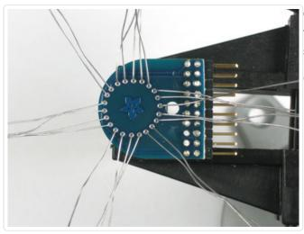
Once you are satisfied, bend the wires out to keep the tube in place and solder each wire, making sure to have no shorts.
