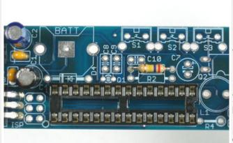
Now place the IC socket. The socket protects the microcontroller chip and allows it to be replaced if necessary.
