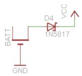
The battery backup is a 12mm lithium coin cells. These cells provide about 3V which is great for running a microcontroller (1.5v is too low). 12mm was used because it was small enough to fit on the PCB but still had enough juice to run the clock (minus display) for a couple of weeks. **D4** is used to prevent the 5V supply from 'charging' the 3V battery, thus destroying it.
