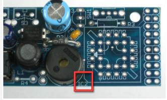
Place the last 0.1uF/100V capacitor **C5** which works with**C7** to smooth out the boost converter
