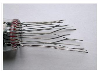
Madworm (http://adafru.it/c1k) suggests cutting the wires in an angle so as to make it easier to place them into the PCB, so you may want to try it!
