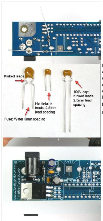
Now place **C1** and **C3**, both 0.1uF ceramic capacitors. Make sure to use the 'plain' 0.1uF capacitors. These **don't** have kinked leads (middle in the lefthand photo).These capacitors are smaller and work with **C2**and **C4**, smoothing out smaller high frequency noise. Ceramic capacitors are not polarized so you can put them in either way!
