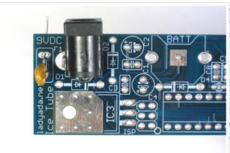
Once you have picked on the correct part, place the fuse next to the jack. Remember it should just fit, if you have to bend the leads a bunch you may have picked out a capacitor. Fuses are just 'wires' so they can go either way and work fine. The fuse protects the circuit, when the circuit tries to draw more than 200mA, the fuse heats up and cuts the power to the circuit. After a whilewhen it cools down, the fuse resets and passes current to the clock again.
