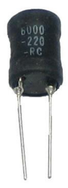
Searching Mouser for power inductors, we find the RLB9012 family (datasheet (http://adafru.it/c1d)) which is the same type used in the mintyboost. This is a good inductor family, lets check out the range.
