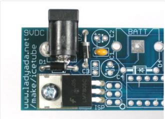
And then lay the part down so it matches the silkscreen. Try to get the hole in the regulator's metal tab to line up with the hole in the PCB. you can make this a little easier by taking a 4-40 screw (such as those in the enclosure kit) and placing it through both holes to line them up.
