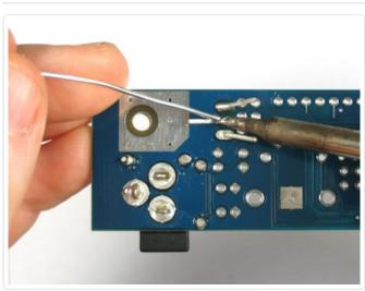
Once you have the 7805 tacked in place, flip over the board and solder in the three pins.
