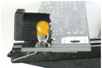
The fuse will sit 'above' the PCB when placed correctly. This makes sure there is plenty of air circulating around the part so dont try and squish it against the PCB all the way
