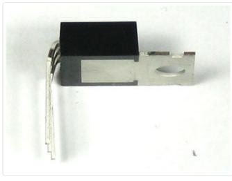
Next is the 7805 5V regulator chip **IC3**. This component takes the voltage from the power adapter, which can be from 7V to 16V, and reduces (regulates) it dow to a nice smooth 5V. Bend the legs into a 90deg angle...
