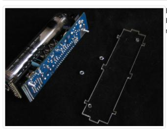
Place two 4-40 screws through the two holes in the PCB from up top, and fasten them with two hex nuts securely.
