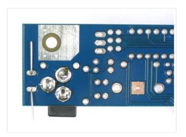
Now using your soldering iron, heat up both the pad and pin of the component and apply solder. Do the same for the other leg.
