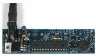
Now we will do another quick test. Clear off the table and plug in the board. You should hear the piezo beep. If it does not, check the 5V regulator, make sure the chip is in right, and that **R1** is in the correct location.
