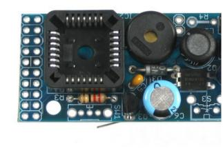
Next place 22 ohm resistor **R3**, this is the bias resistor for the VFD tube heater. The resistor is symmetric.
