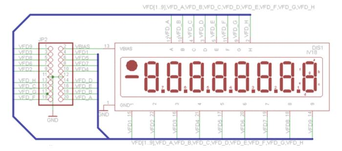
The VFD tube is the display for the clock. It has 9 digits, 8 of which are standard 7 segment plus dot displays. The leftmost digital has only a \* and -. Instead of having 60+ connections for each segment, the display is gridded out so that you can only turn on one digit at a time (1-9) with the selected segments (A-H). The microcontroller sweeps through all of the digits in order at >100Hz so that it appears as if they are all lit up at once.
