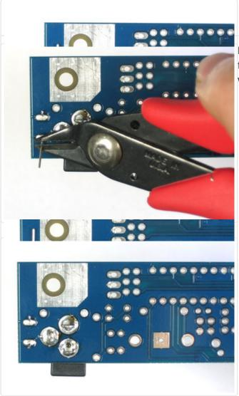
Next it is time to clip the extra long leads of the fuse. Using your diagonal/flush cutters, clip the wires right above where the solder joint tapers off.
