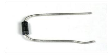
supply (backwards) which would make the kit release its 'magic smoke'. As you can imagine, its important to place the component in the right way. On one end of the diode is a white/silver stripe. Make sure this stripe matches the stripe in the silkscreen image. See the image left if you're not certain.
