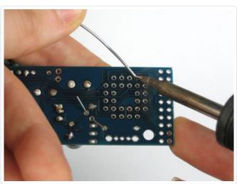
Once you are sure you have done it right, flip the board over and solder in all the pins of the socket and the capacitor.
