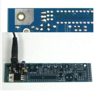
Now is a good time to take a break and test your work so far. Place the board down on a clean surface - make sure there are no stray wires or solder balls, etc.
