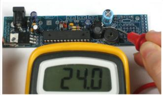
Unplug the DC jack and continue to measure the voltage on the diode. It will slowly drift down. When it is around 15VDC you can continue to work on the kit.
