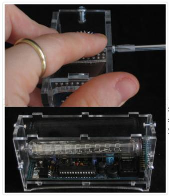
Stand the clock upright. Insert the last two 4-40 screws and hex nuts into the sides if you havent yet.
