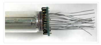
Before soldering, do a test by plugging the tube into the mainboard. Tubes vary a lot and some are bent a little. Make sure that tube is straight with respect to the main PCB. You can pull the tube a little to angle it so that it ends up straight.
