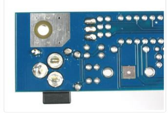
Next is **C2**, the 47uF/25V electrolytic capacitor. This capacitor smooths out any large ripples in power coming into the kit. Electrolytic capacitors are*polarized* which means they must be placed correctly or they wont work at all. If you look at the capacitor you'll notice one leg is longer than the other, this is the positive (+) lead. Make sure this lead goes into the pad silkscreened with a +. See left for how to place the capacitor.
