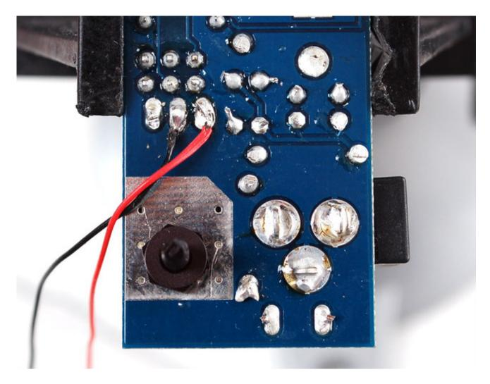
Connect the TX wire of the GPS to the RX pin of the microcontroller (pin 2).
