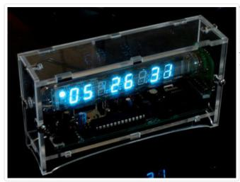
You're done! Now its time to make the enclosure. Do not operate the clock without an enclosure! An insulating enclosure is essential to protect the user from accidentally touching the high voltage on the VFD display.
