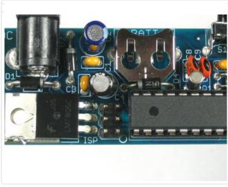
Finally, if you're planning to ever ugrade the firmware or hack the clock, solder in the ICSP header. The longer pins go on top.
