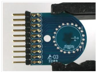
Finally solder in the rest of the pins.
