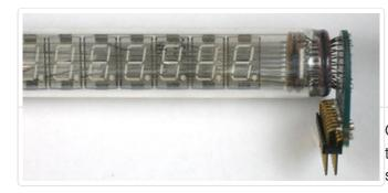
Once you are satisfied, bend the wires out to keep the tube in place and solder each wire, making sure to have no shorts.
