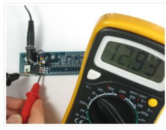
Now find your handy multimeter, and set to measure DC voltages (and set the range if necessary).
