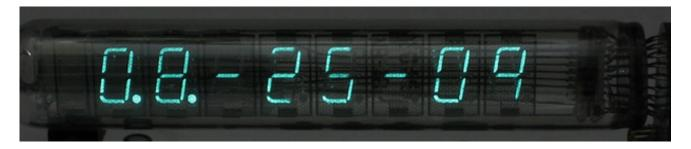
Press the + button to change the month. You can hold down + to quickly spin through the numbers.
