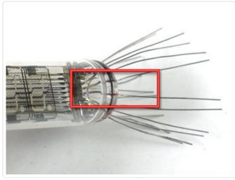
connected wires. in this case, the spacing will be different in front and you'll see two wires that seem 'farther' than the others. They are right in the front of the tube and are the two pins in the 'middle' of the front plate (which has 4 connections). Make sure you have identified the correct wires, please click the photos to the left to see larger detailed images as its much easier to see than explain.
