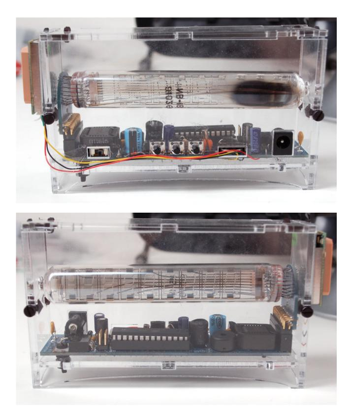
OK turn on the clock and you will find the GPS blinking. The time will likely be wrong so stick the clock near the window until you see that the time **minutes** are correct (the hour will still be wrong).
