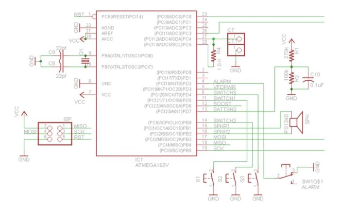
Finally we get to the brains of the project, an AVR microcontroller. This one in particular is the ATmega168V or 168P. The V or P designation means it can run at 1.8V voltages, otherwise the chip requires 4V or more to run and that is more than the battery backup voltage
