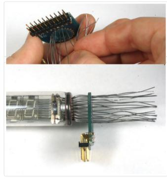
Straighten out the wires with pliers and slide the tube down. This will take care and patience as the wires are thin and bend easily. Work slowly and use pliers to gently pull on any kinked wires.
