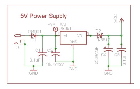
The first part of the circuit is the 5V power supply. This is a generic 7805 style circuit.
