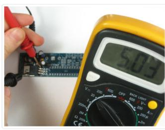
Now check the 5V regulator by probing the third pin (closest to the 'top' in this image). You should get a steady voltage between 4.7V and 5.2V DC
