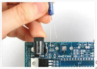
Once the electrolytic capacitors are placed correctly, bend out the leads and solder them in place.
