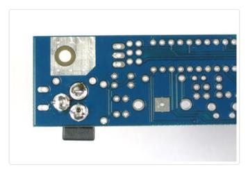
The second part to go in the fuse**F1**. The fuse looks suspiciously similar to a ceramic capacitor. So before you continue lets identify the fuse.
