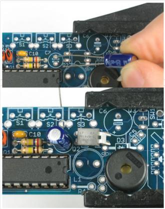
We also need to place the high voltage transistor that does the switching in the switching regulator. Its a little confusing how to place it because there is no notch. However, two of the pins are bridged. These go on the right as shown.
