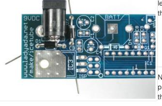
Now using your soldering iron, heat up both the pad and pin of the component and apply solder. Do the same for the other legs.
