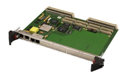
connectors. Another two Gigabit Ethernet channels are available at the optional P0 rear connector to support Ethernet on the backplane complying with ANSI/VITA 31.1-2003.
