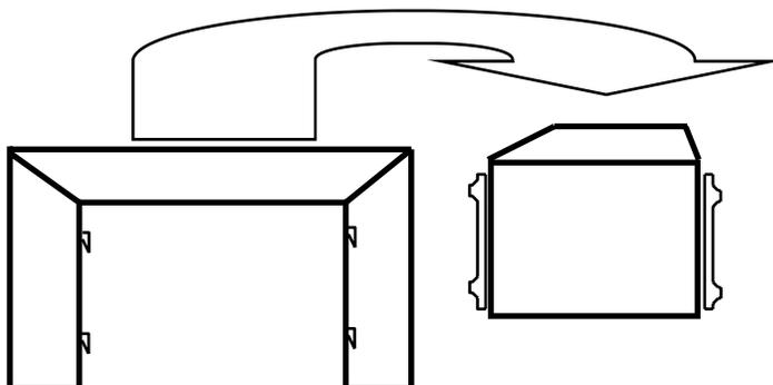
The surround has four hooks that clip onto the sides of the appliance. Make sure the surround sits evenly with the front of the fireplace. After the surround is properly installed, the bottom edge of the centre section of the surround is about  $\frac{3}{4}$ " from the top of the appliance.
