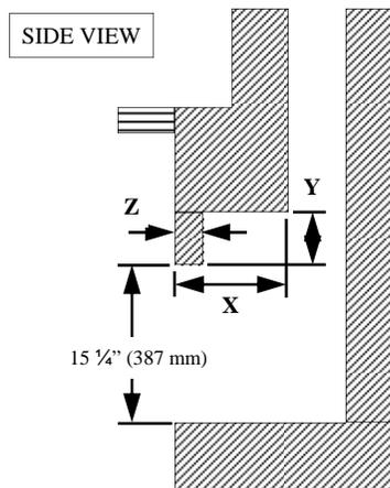
The standard flue adapter will fit if **X** is more than 5 3/4". It will also fit if **X** is less than 5 3/4" but **Y** is higher than 8" (See 'Flue connector, offset vent' diagram)
