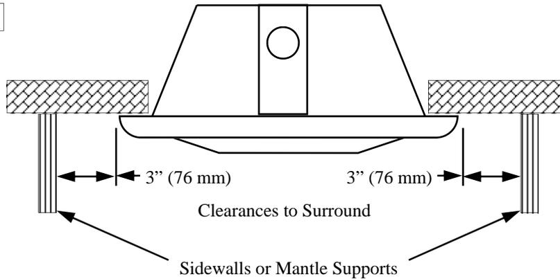
**CAUTION:** This appliance is designed for use in any masonry, factory-built wood burning and specific zero-clearance vented gas fireplaces (Due to constant additions, contact Archgard Industries for an updated list of suitable gas fireplaces). This appliance cannot be enclosed with combustible material and used as a built-in gas fireplace.
