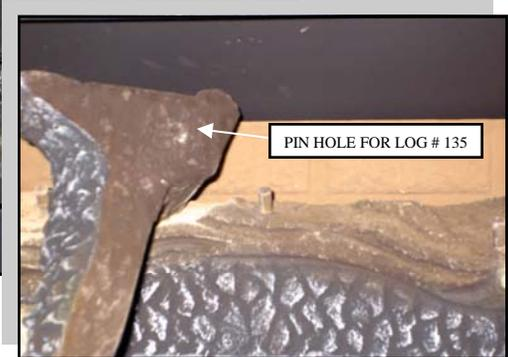
**STEP 7** - Locate log #139 and place onto rear log using the locator pins and pre-drilled holes in log. Log should sit behind right grate tine as shown in photo below.
