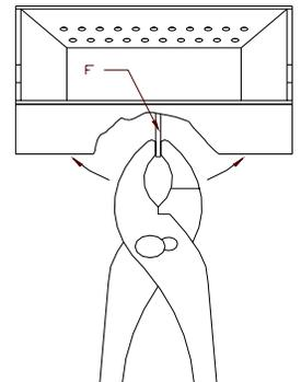
Grasp the burn grate adjustment tab (F), with a pair of pliers and bend it slightly to left or right (and re-install into burn box) until its length allows the burn grate top to rest tightly onto the burn grate bottom. (Location J)
