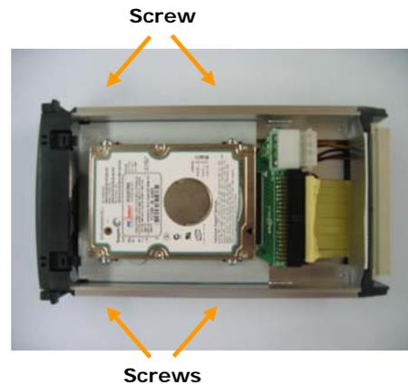
4. Attach the Bracket onto the Tray by using the supplied screws and insert the Tray into the DVR HDD slot.
