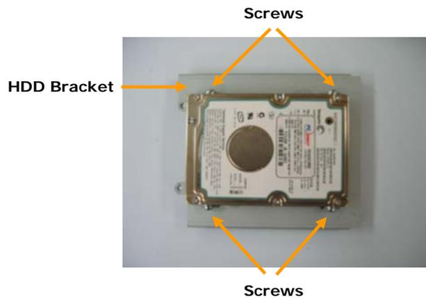
2. Detach the HDD Bracket from the Tray and attach the 2.5" HDD onto the Bracket with the supplied screws.
