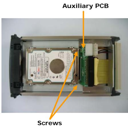
3. Insert the HDD Bracket into the Tray and connect the 2.5" HDD to the Auxiliary PCB. Then fix the Auxiliary onto the Bracket with the supplied screws.
