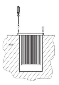
Connect the fixture to DC power supply or driver and put the fixture in the box. Fit the top of luminary with screws in.
