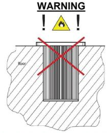
The fixture never input directly into the ground without any floor box.
