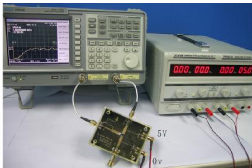
[Fig.9-6] Measuring Characteristic of PIN Diode Switch
