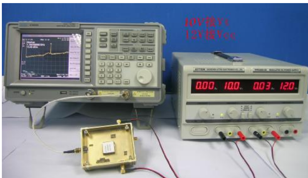
[Fig. 1-9] Output measurement of VCO
