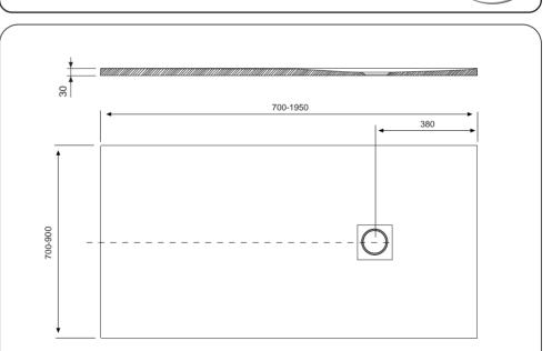
The dimensions of the shower trays have a tolerance of + /- 2,5mm.
