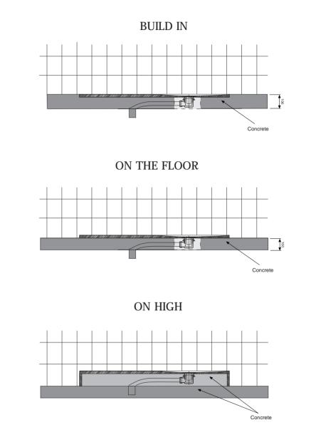
NOTE: On high installation the shower-tray has to be installed on a leveled and smooth surface too. This surface have to cover all the shower-tray's surface.
