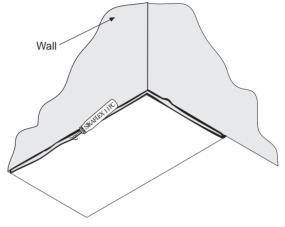
Apply a thin and uniform layer of flexible polyurethanemastic to secure the fixing of the shower tray.
