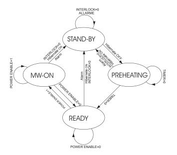
**READY:** it's a waiting state, the display shows "RDY". The unit waits the enabling command to generate power to the magnetron. The magnetron filament has been heated. The unit may last in this state as long as needed: it exits automatically in case of alarms or when the" filament heating" command is removed. It goes to next "MW-ON" when the enabling command is set ON.
