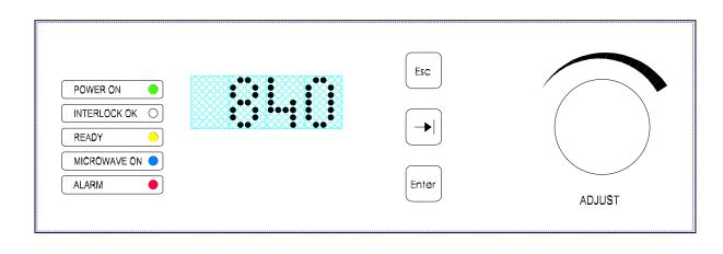
c) in ON state -and HIBERNATE is OFF- the unit wait the end of preheating timer, if not yet elapsed, then starts to generate output power;
