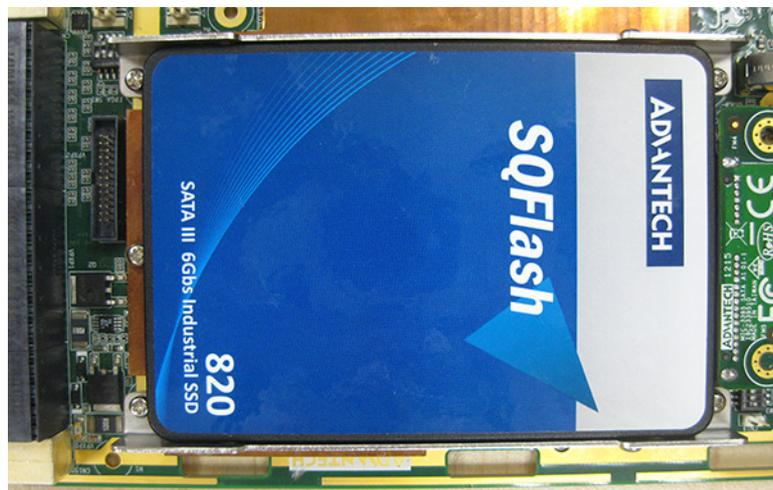
**Figure 1.7 Inserting the SATA HDD into the SATA connector**
