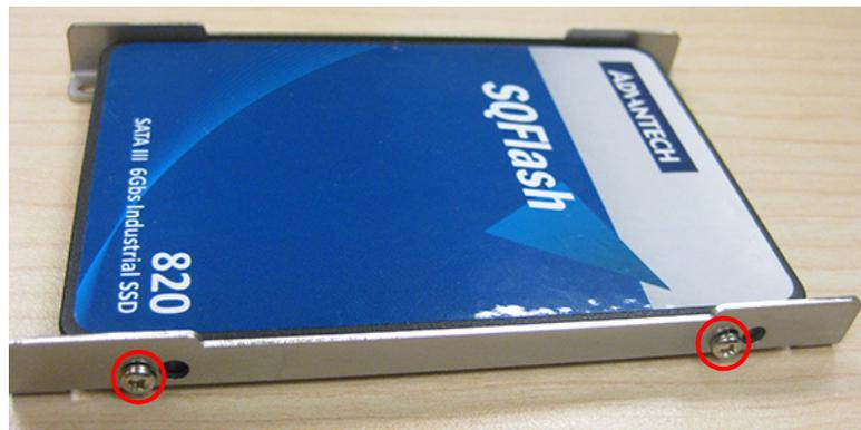
**Figure 1.6 Fastening screws to the SATA HDD bracket**
