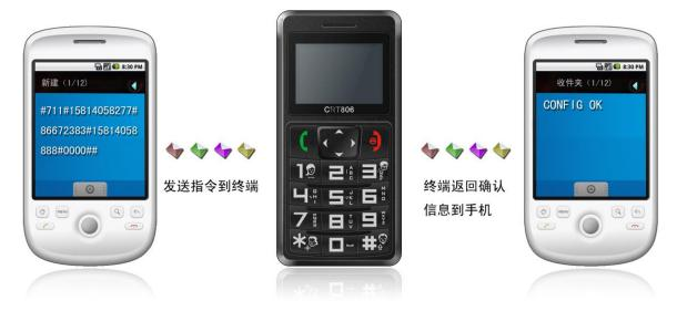
Send command to the terminal The terminal will return confirmation message to the mobile phone Description: After the setting is successful, press the SOS key, then the terminal will circularly dial the set phone until it is connected.
