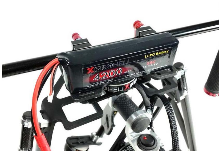
Connect the provided banana to 3-way male JST adapter harness to the battery. One of the 3 male leads will be used to provide power to the Silk. The other two leads can be used to power a light set or a on board monitor (12v out).
