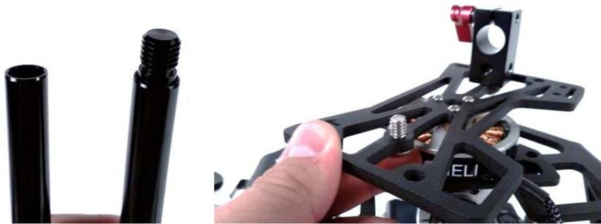
Mount the (2) 15mm rod clamps to the top plate of the Silk. There are several sets of through holes to choose from, it is most common to mount the rail clamps to the holes aligned at the center of the motor.
