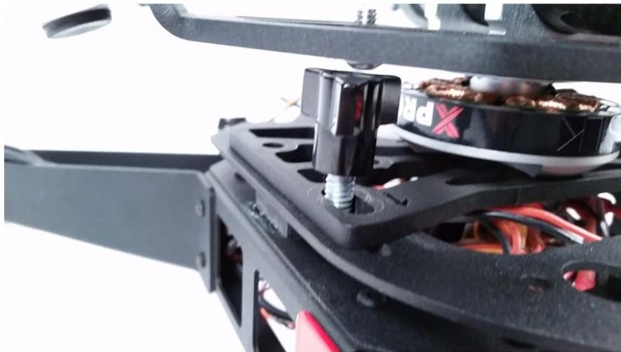
Connect your power wiring from your DC to DC down-converter (BEC) or 3S power source and connect any desired remote tilt wires to the control box from your receiver – This is typically setup on AUX 3 output port of your AR8000 receiver and controlled on the FLAP switch of your DX8 radio.
