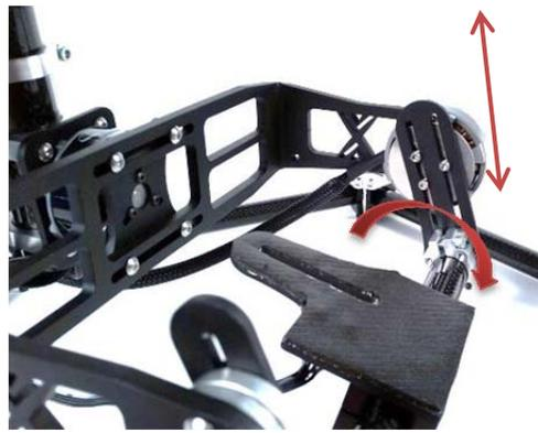
**Hint:** The Silk is considered balanced when the camera remains static in all positions and cannot fall to either side of any axis. If the camera is not perfectly balanced the gimbal will still work very well, but it will cause the motors to work harder. Best stabilization performance is achieved when you have a perfectly balanced gimbal.
