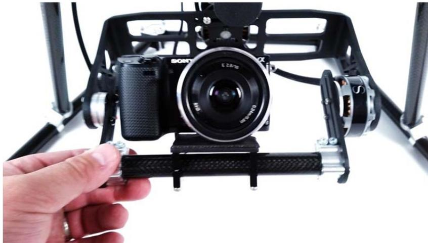
Adjust your camera's center of gravity on the pitch and roll axis by loosening the set screws so that you can slide the assembly in the opposite direction of the weighted side to balance the camera.
