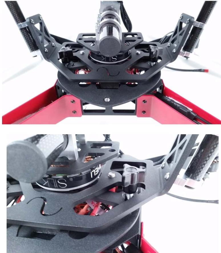
Connect your power wiring from your DC to DC down-converter (BEC) or 3S power source and connect any desired remote tilt wires to the control box from your receiver – This is typically setup on AUX 3 output port of your AR8000 receiver and controlled on the FLAP switch of your DX8 radio.
