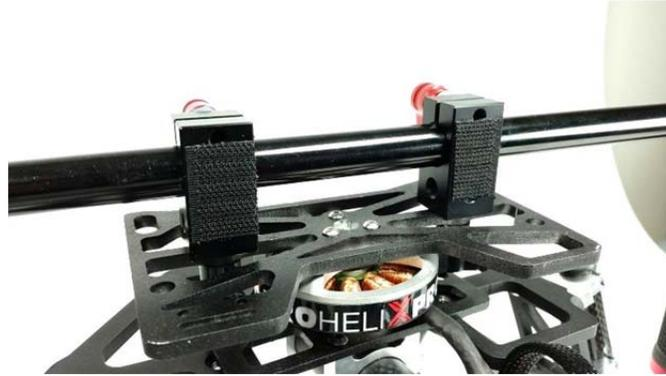
Your battery pack (4200mah XPH 3S) comes with a strip of long sided Velcro. Mount the battery pack horizontally to the back of the clamps as shown:
