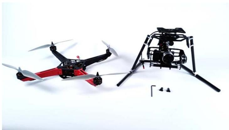
You can mount your XPX airframe to the Silk in an upright configuration, however we recommend mounting the Silk to the airframe upside down to help align the Silk centered on the XPX. Line up the two through slots on the front of the top plate and fasten the mounting plate using the ¼-20 toggle screws to the left and right lander pem nuts on your XPX:
