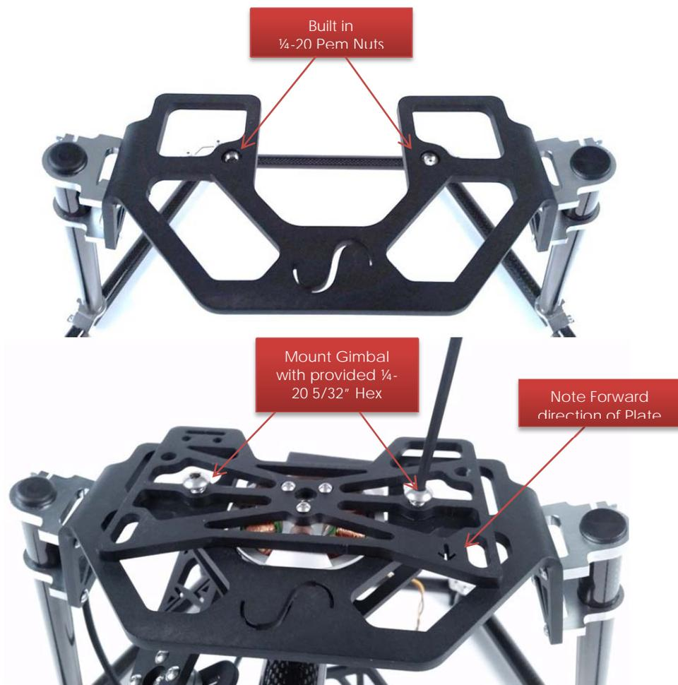
Depending on your mounting preference or mode of operation with the Silk (i.e. 2<sup>nd</sup> operator) you also have the option of mounting the gimbal to the stand using the lower plate as shown below. This plate is also used to 'rest' the gimbal on the stand when used for handheld operation.
