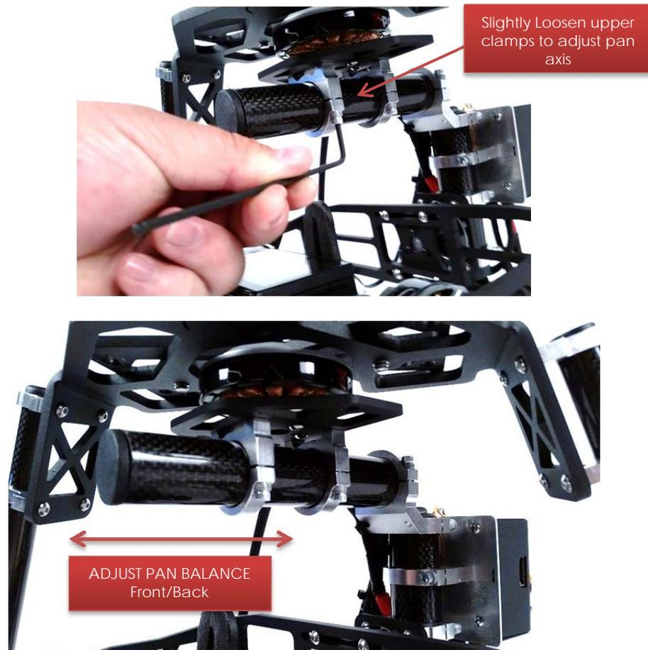
Adjust the pan axis similar to the roll and pitch axis by holding up the top pan axis plate at a 90 degree angle. If the pan axis is weighted to far to the left or right side or weighted to far forward or too far back it will fall to the weighted side. Adjust this by sliding the tube inward or outward for front to back balance and rotating the tube left to right for side to side balance. A perfectly balance pan axis will hold position by its self in all 360 degrees of motion.
