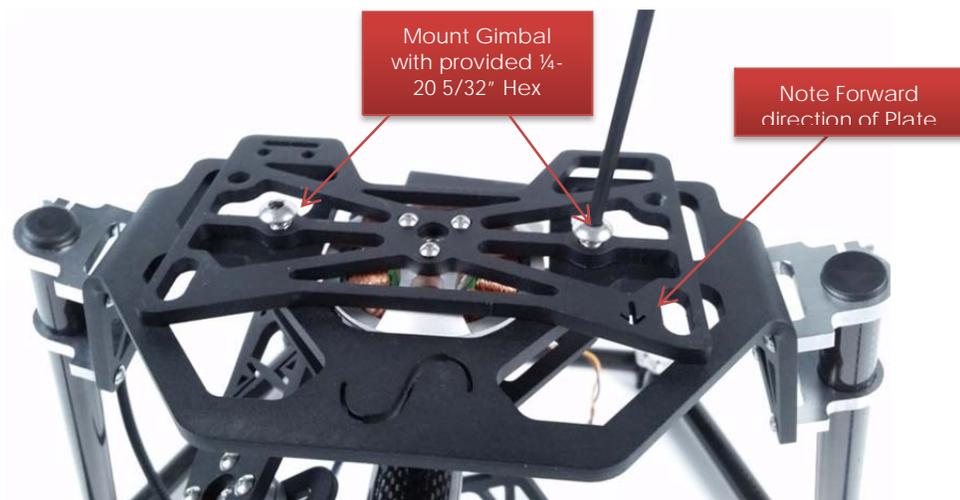
You can mount your XPX airframe to the Silk in an upright configuration, however we recommend mounting the Silk to the airframe upside down to help align the Silk centered on the XPX. Line up the two through slots on the front of the top plate and fasten the mounting plate using the 1/4-20 toggle screws to the left and right lander pem nuts on your XPX:
