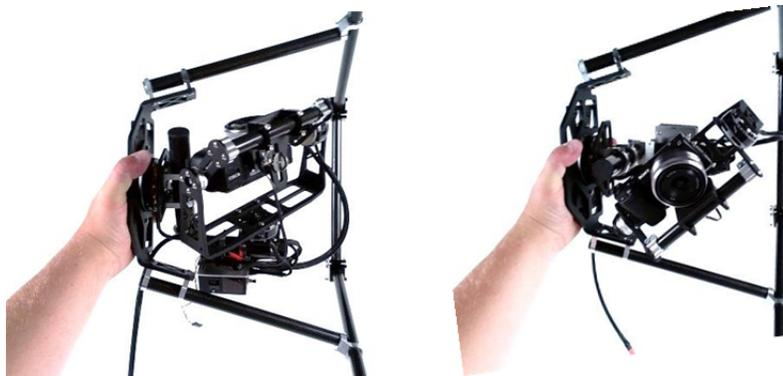
If you find that the pan axis seems to be balanced in some positions but in others it tends to fall to the left or right side of the camera then you need to make a further adjustment by rotating the top carbon fiber tube either left or right to counter balance the heavy side.
