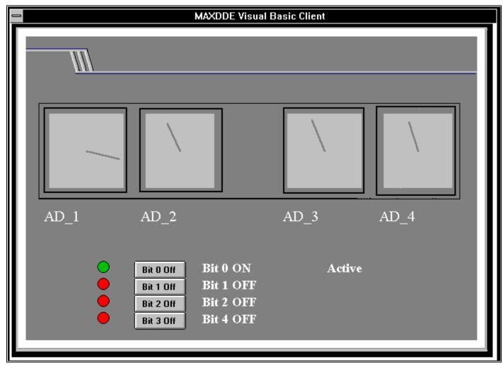
The Visual Basic program developed lets the user set bits via the **Bit 1 Off** through **Bit 3 Off** keys. When pressed they say **Bit 1 On** through **Bit 3 On**. The text to the right of the buttons tells the status of the input bits and the "LEDs" the left of the buttons turn RED when an input is OFF and GREEN when an input is ON. The gauges are Visual basic controls. There is a bit map backdrop for the whole form that would have the markings for the gauges given units of measure etc.
