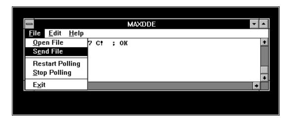
The **Send File** menu option lets you select a .FTH file and send it to a node on the EASY-A network. The download is done following the appropriate text transfer protocol. (Wait for echoed character, send the next line upon reception of a linefeed.)
