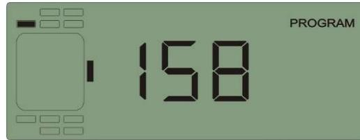
7. When finish programming these 3 digits, press S for 3 seconds to save with the screen flashes twice, beep buzzes twice. Then it will automatically switch to next tire position.
