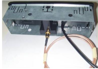
1.3 Fix antenna and antenna mounting bracket with 2 pieces of 3M Dual Lock Fastener
