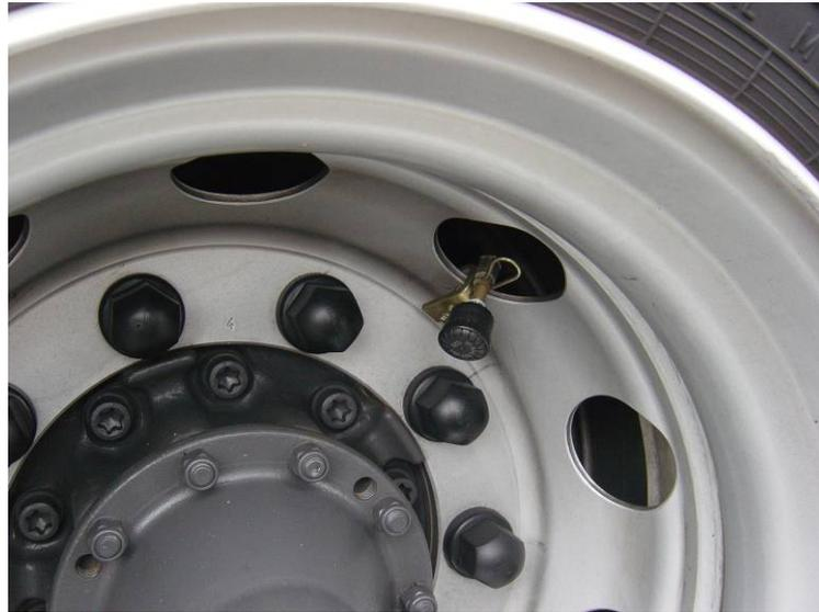
1. Remove the current tire valve cap.
