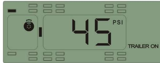
Function: The system will issue a fast leak alarm when the pressure drops more than 2.8 psi within 12 seconds.
