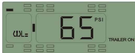
Function: The system will issue level 2 low pressure alarm when the tire pressure is 10% lower than the standard pressure.
