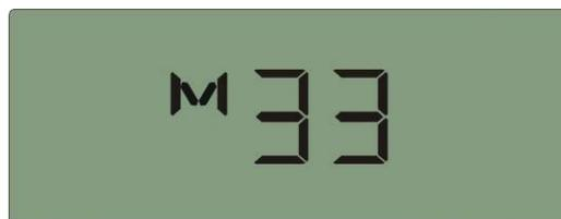
Under any interface of system time inquiry, press S for 3 seconds to start programming. For example change the year to “09”, under the “year” interface, press S for 3 seconds, the second digit flashes, press up or down key arrow key to adjust the value. Then press
