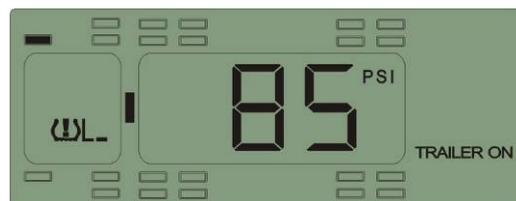
Function: The system will issue level 1 low pressure alarm when the tire pressure is 5% lower than the standard pressure.
