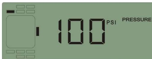
3. Then press S for 3 seconds to set the first digit which flashes. Press up or down arrow key to adjust the value to 1.
