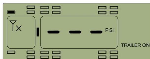
Function: If one transmitter fails to work, or the monitor cannot receive the data because of the RF interference for 20 minutes, the system will issue a transmitter trouble alarm.
