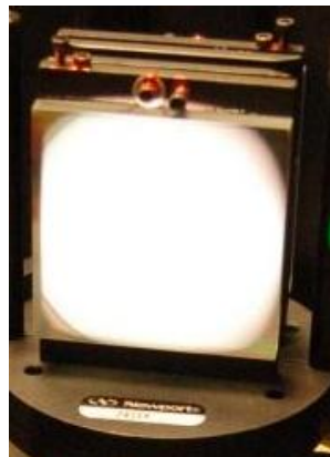
Figure 20: Grating Correctly "Filled" with Light
