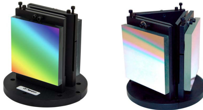
Figure 14: Gratings Installed onto Mounts
