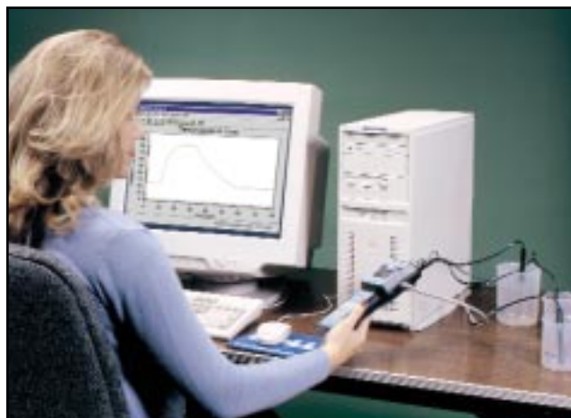
Figure 2 Measure and log the conductivity of water samples.
